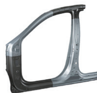
Integrally molded door ring
