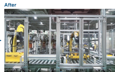
Saitama Plant fully automated welding line (patent no. 7261929)
