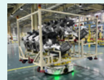
Automated transportation (AGF/AGV)
